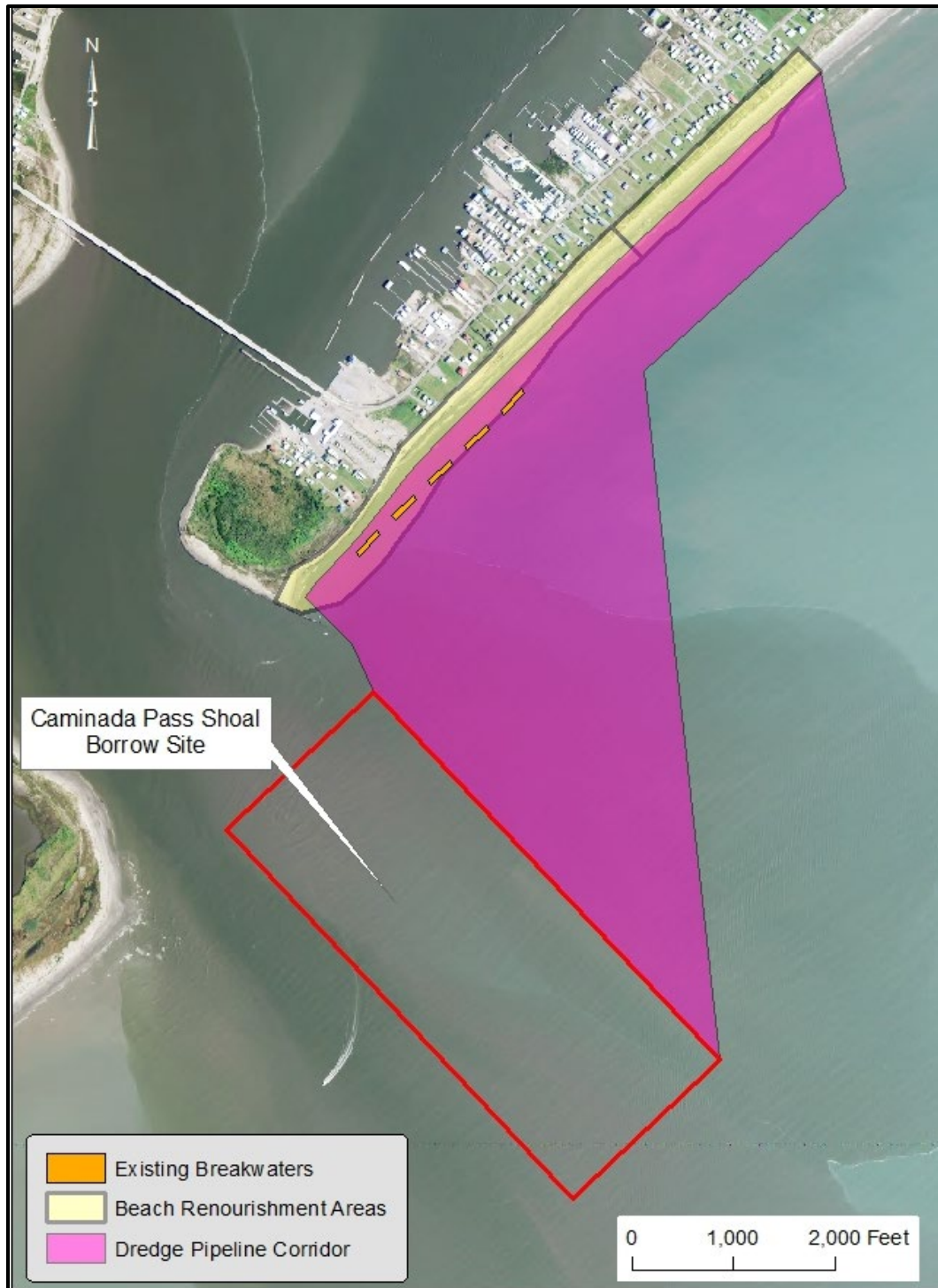
Figure B4. Proposed dredge pipeline corridor extending from the proposed Caminada Pass Shoal borrow site to the proposed beach renourishment and Dune Restoration areas.
